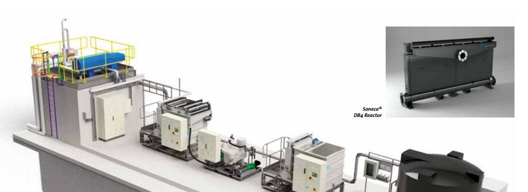
With a small physical footprint, Soneco® is easily integrated or retro-fitted to existing over-loaded or under-performing works, and sludge volumes are up to 40 per cent lower than with other methods. The system is eco-friendly and has a greatly reduced environmental impact and improved carbon footprint.
