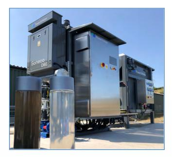
As specialists in the latest generation of innovative water treatment technologies, Power & Water (P&W) were invited to meet representatives from the facility after sample testing at our in-house laboratory proved effective. The aim of which was to discuss the potential of using P&W's patented Soneco® treatment process, utilising sono-electrochemistry to reduce the elevated levels of contaminants produced from the facility Penmon, Anglesey.
