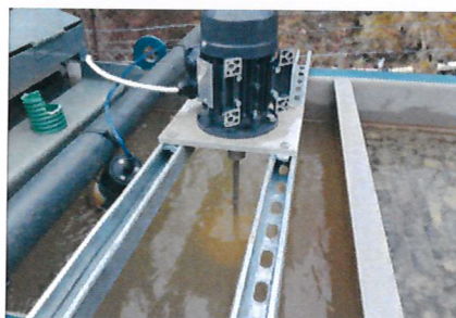
Above: Floc on clarifying tank at Cwm Rheidol after set-up Below: Tank after optimisation, with stirrer fitted
